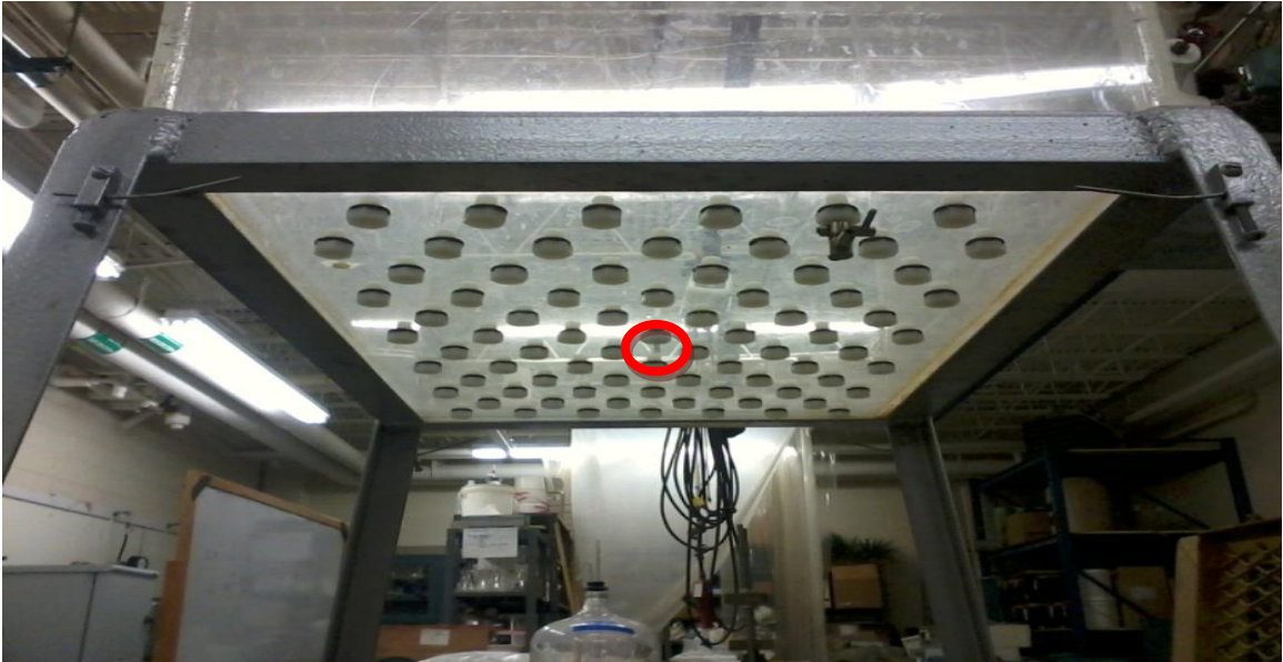
Figure 3.2: The smaller gravity-fed rainfall simulator with the single dripper circled near the center of the simulator
