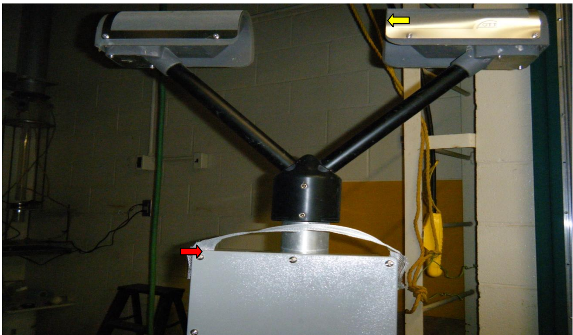
Figure 3.10: Wire mesh placed on the upward-facing portion of the power supply box, indicated by the right-pointing arrow. The flange was located at the end of the left-pointing arrow.
