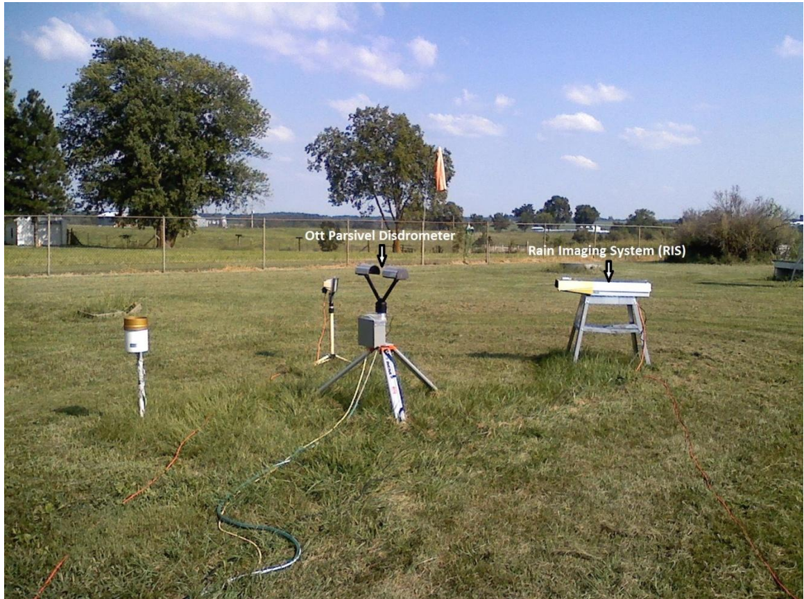
Figure 3.4: Setup for data collection at South Farm including the Campbell Scientific rain gauge, OTT Parsivel Disdrometer and the Rain Imaging System.
