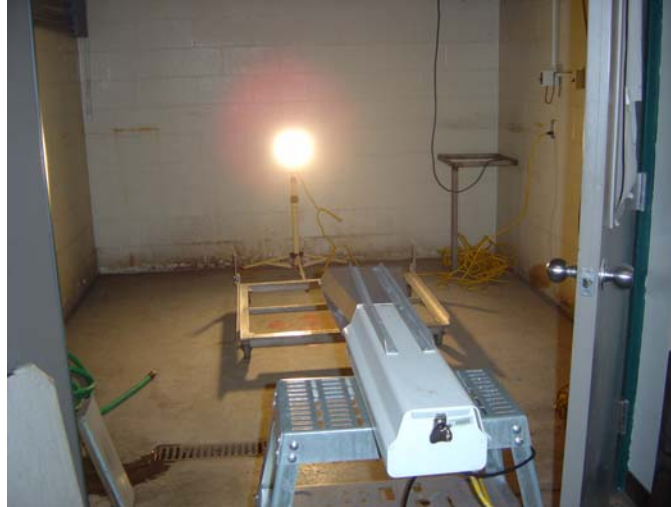
Figure 3.8: Deployment of the RIS in the Hydrology Laboratory where simulated raindrop data was gathered.
