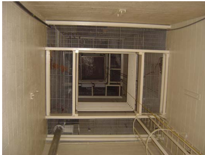
Figure 3.9: View looking upward showing the vertical extent of the indoor rainfall simulator located in the Hydrology Laboratory.
